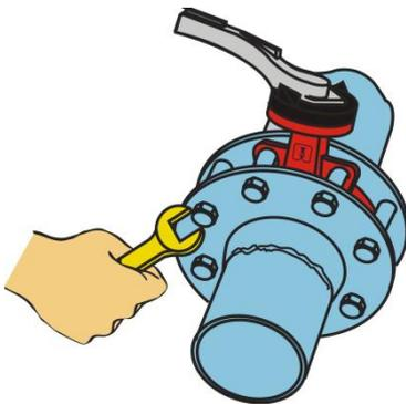
9. Add the remaining bolts and tighten them firmly (in a "criss-cross pattern").
