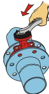
6. After the flanges have cooled down, insert the valve, and ensure sufficient clearance (see Fig. 1).
