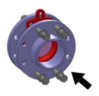
2. Tighten the flanges lightly with four bolts and align the position of the valve.
