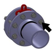
7. Centre the valve and tighten it lightly using four bolts. Add the remaining bolts (tighten them in a "criss-cross pattern").
