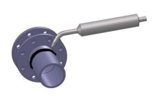
5. Weld the flanges to the piping.
