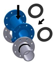
6. When the flanges have cooled down, insert the filter again with gaskets. The arrow on the body must coincide with the flow direction.
