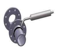
5. Weld the flanges to the piping.
